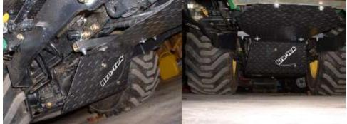
For those of you, that wants to protect the fuel filter/pump & expose wiring, the front skid plate extension is seen on the above photo.
