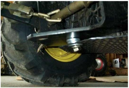
Install the two spacer & nut/bolt. Use a 15/16"
